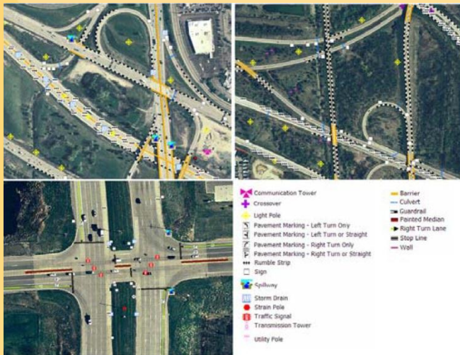
Figure 1: An example of an intensive road furniture inventory collected using the imagery-based methods captured in the Road Furniture Desktop GIS Tool.
