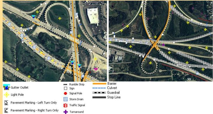
**Figure 1:** Examples of “road furniture” asset management data collected by application of high-resolution imagery; the analysis and data collection process is now captured in a user-friendly desktop GIS tool developed under the TARUT study.
