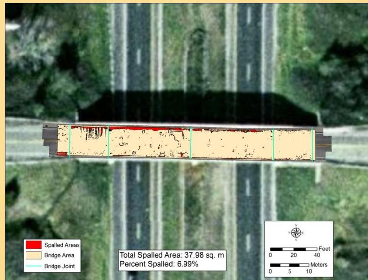
Figure 4: Automatically mapping spalls on bridges using 3DOBS data.
