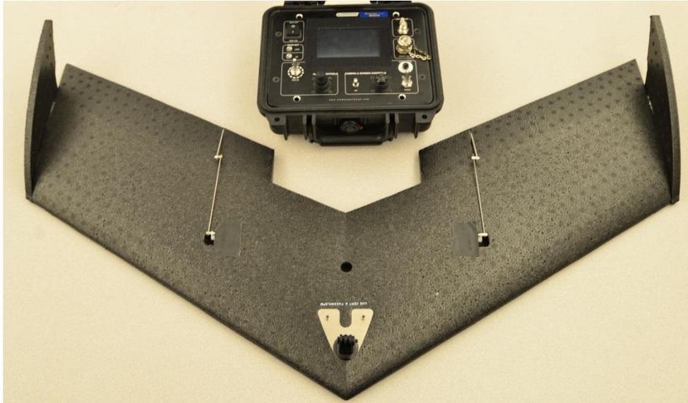
**Figure 3-2: Lehman LP-960 wing and ground control station.**
